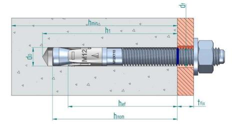
$\begin{array}{ll} d_0: & \text{Nominal diameter of drill bit} \\ d_f: & \text{Fixture clearance hole diameter} \\ h_{ef}: & \text{Effective anchorage depth} \\ h_1: & \text{Depth of drilled hole} \end{array}$
